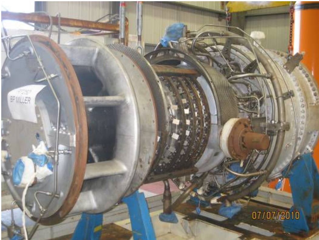
Siemens SGT-200 (Tornado) Dual Fuel Industrial Gas Generator
