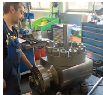
Overhauled ball valve (4 1/16" PN 520) during re-assembly at Hartmann factory
